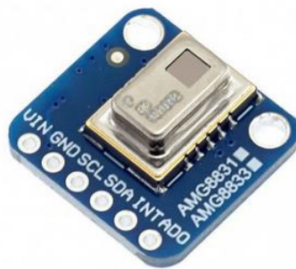
Figura 9. Sensor IR 8x8 AMG8833 Panasonic. (Mechatronics, 2021)
