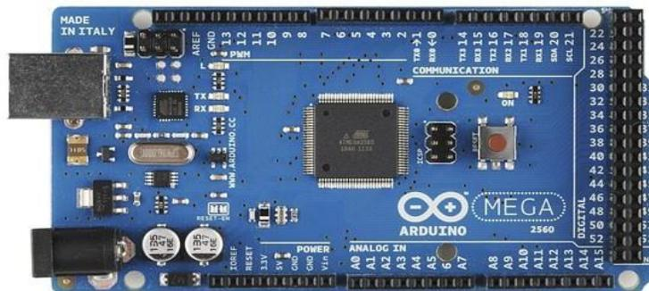
**Figura 22** Arduino MEGA
