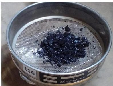
Figura 1. Tamiz Dirimpex #20 Fuente (Autor)
