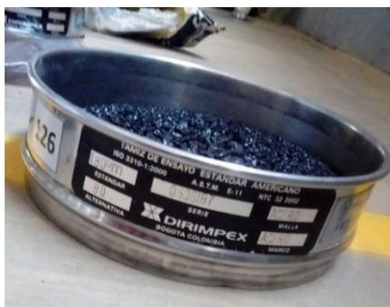
Figura 2. Tamiz Dirimpex #80 Fuente (Autor)
