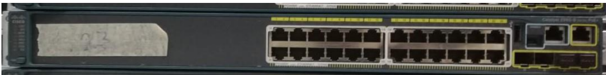
Figura 22. Switch Cisco 2960-s
