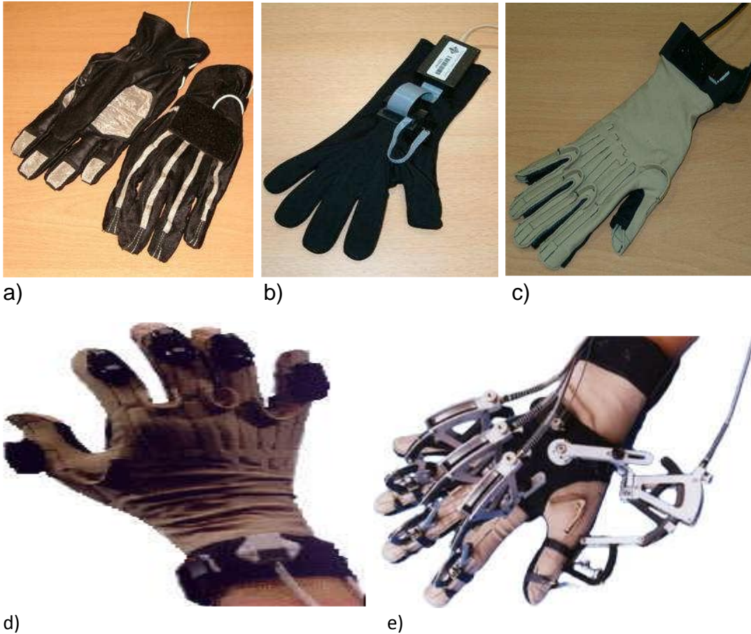
Figura 4. Guantes de datos. a) FakeSpace Pinch Gloves b) Fifth Dimension Data Glove c) Immersion CyberGlove d) Immersion CyberTouch e) Immersion CyberGrasp.
