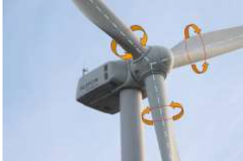
Figura 44. Control de pitch [www.wtindustries.com]
