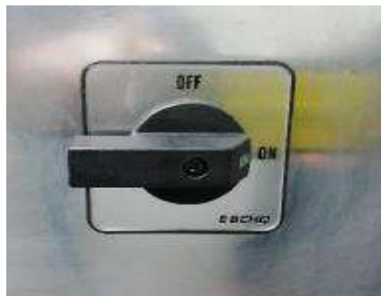
Figura. (7.7) 16: Selector principal en modo ON.
