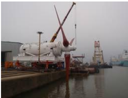
Figura 7. Turbina Andritz Hydro HS 1000 (Hydro, 2012).
