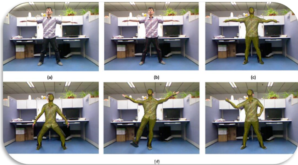
Figura 2 10 (a) User in Kinect RGB video stream. (b) Rectified skeleton using inverse kinematics (IK). (c) Tracking result for user shown in (a). (d) Three more tracking results under the movement of limbs. (Jiang, Zhao, & Liu, 2014)
