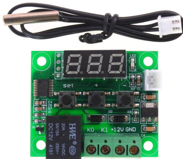
Figura 33 Minitermostato digital w1209 (“W1209 TEMPERATURE CONTROL SWITCH,” n.d.)
