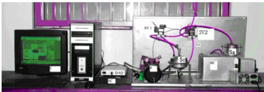
DAQ: data acquisition card SC: signals conditioner P: vacuum pump Sa: sample chamber Sc: sensor chamber SV: solenoid valve HC: heating chamber.
